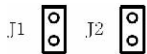
(a) J1, J2 open circuit PUL/DIR mode and effective at upward-rising edge
