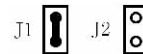
(b) J1 short circuit, J2 open circuit PUL/DIR mode and effective at downward-falling edge
