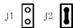
(c) J1 open circuit, J2 short circuit CW/CCW mode and effective at upward-rising edge
