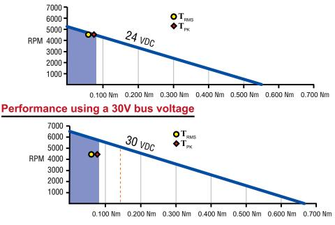
A 30 VDC bus will meet the application requirements as wells supply a margin of safety.
