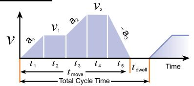
Linear Motion Formulas (1)  $S = \frac{V_f - V_i}{2}t$ (2)  $V_f = V_i + at$ (3)  $S = V_i t + \frac{1}{2} at^2$ (4)  $2aS = V_f^2 - V_i^2$ (5)  $a = \frac{(V_f - V_i)}{(t_f - t_i)} = \frac{\Delta V}{\Delta t}$ Linear to Rotary Formulas - through a Lead Screw  $\mathcal{Q} = \frac{2\pi a}{L} = rad/s^2$ (1)  $\mathcal{Q} = \frac{2\pi V}{L} = rad/s$ (2)  $\mathcal{Q} = \frac{2\pi V}{L} = rad/s$ (3)  $\mathcal{Q} = \frac{2\pi V}{L} = rad/s$ (4)  $\mathcal{Q} = \frac{60V}{L} = RPM$
