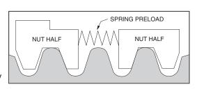
For example, if the maximum axial load to which the system is subjected is 50 lbs., the amount of spring preload must be equal to, or greater than, 50 lbs. in order to maintain intimate screw/nut contact. The problems arising from preloading in this manner are increased drag torque and nut wear.
