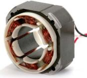
The slotless design also reduces damping losses related to eddy currents. These currents are weaker in a slotless motor, because the distance between the laminated iron and magnets is greater than in a slotted motor.
