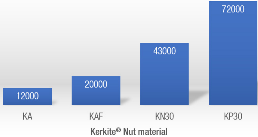
Fig. 2: Kerkite® Composite Polymers offer wide range of PV values
