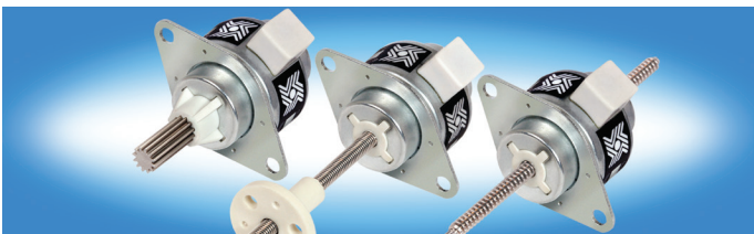
Figure 10. CAN-STACK LINEAR ACTUATORS G4 25000 Series: (Ø 1-in / 25.4 mm) captive, external linear, non-captive available in 15 and 7.5 rotational degrees per step.
